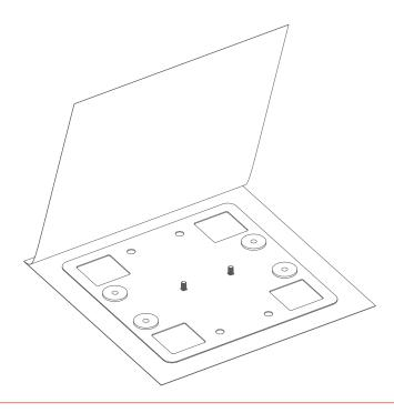
Install the M10 bolts and washers in the plate, connect it to the bar and arrange it in the desired place on the roof. Tighten the nuts with a torque of 36Nm, which will ensure tightness between the base of the bridge and roofing felt.
