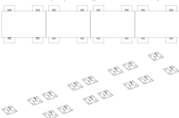
Cut the membrane/roofing felt to size 510x510 mm. Make holes for the lock bolts. Weld the membrane/roofing felt at four fixing points and 50 mm around the fixing plate.
